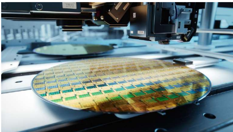
Fig.1. Semiconductor silicon wafer undergoing probe testing during chip manufacturing. Source: iStock/Getty Images, image ID 887333134 (genkur, 2017).
